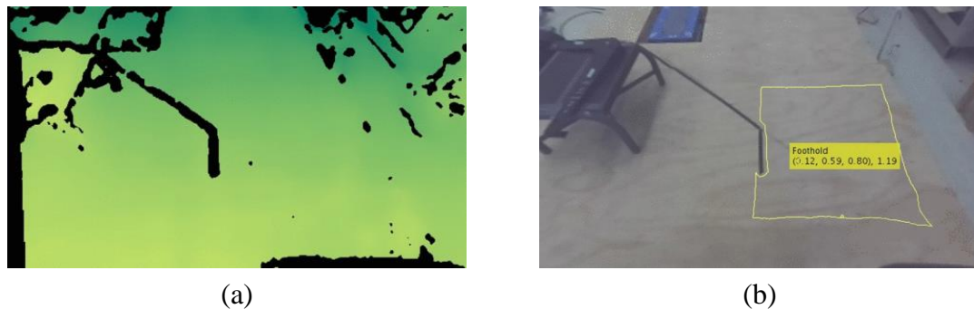
Figure 4. (a) Depth map from the image capture. (b) Selected region of interest for the ground plane estimation.
